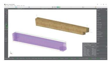
The cadwork 3D engine offers many possibilities to import data from other software, in the most common formats (DXF / DWG, SAT, etc ...) as well as the best performance formats (IFC). You can get and use some three-dimensional volumes ready to be converted into machine data.
